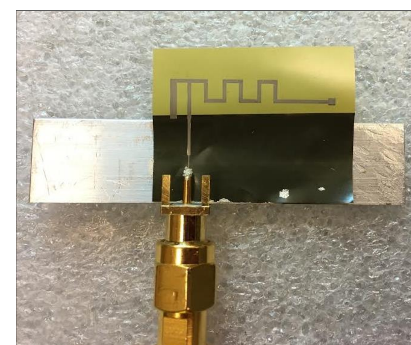
Fig. 7 Printed Inverted F Antenna mounted for testing.
